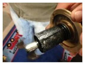
Magnetite gets into tight spaces such as valve seats and packings, and wetted bearings, for example, where friction can cause wear, seizing, leaking and mechanical failure.
