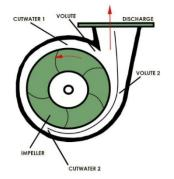
Almost all hydronic systems have at least one wetted component made of cast iron or steel such as pump volutes<sup>2</sup>, expansion tanks, etc.
