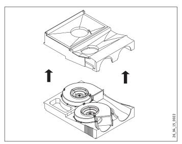
► Carefully remove the top EPS insulation semi-shell so that both fans are accessible. Ensure that the fans remain in the lower EPS insulation semi-shell.
