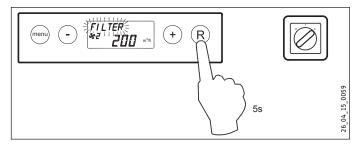
► After cleaning or replacing the filters, hold down the R key for 5 seconds to reset the filter display.
