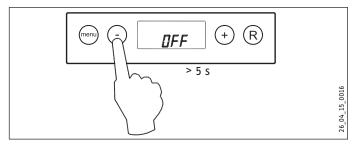
► Switch on the appliance by pressing the minusbutton for 5 seconds.
