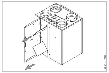
► Extract the supply air and extract air filters. Make a note of how the filters were fitted.
