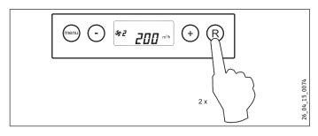
If no key is pressed for 5 minutes, the appliance returns automatically to standard mode.
