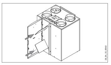
▶ Push the cleaned or new filter into the appliance.
