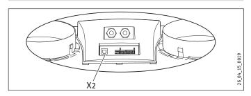
Connect the stage switch (not part of standard delivery) to the modular plug-in connection, type RJ12 (X2 connection). The X2 connection is on the back of the appliance's display cover.
