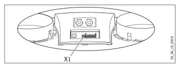
To connect an eBUS or OpenTherm connection, there is a 2-pole X1 connection on the back of the display cover.
