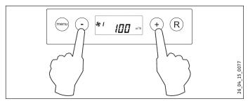
All display symbols light up for three seconds. The appliance is then in standard mode.
