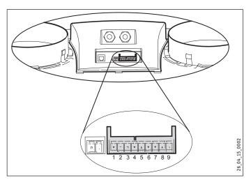
The 9-pole X15 terminal strip can be accessed on the back of the display cover without having to open the appliance.
