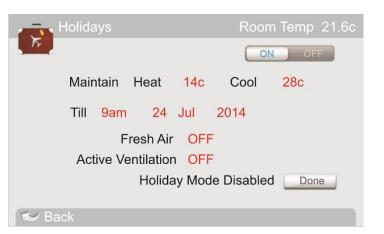
return. Then simply select ON. The Falcon will open all zones and control your heating and cooling system to maintain your desired temperatures as measured at wall controller 1.
